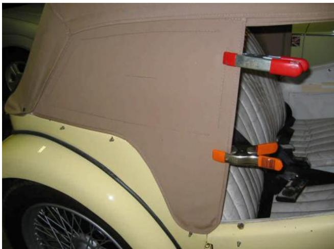
own. Now use a chalk pencil to trace around the inside of the frame, marking the fabric cover, while it is on the car. Next issue, we will look at punching the cover, cutting out the fabric and choosing/installing the outer frame pieces. Who knows, maybe we will finish this project before the next dry spell!
