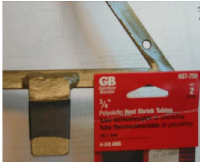
The next step will be to bend the new frames to conform to the shape of the car because they arrive welded-up in dead-flat geometry. Starting on one side of the car, fit the rear frame and adjust the attachment plate with stud, if necessary, to provide a good, preliminary fit. I slipped on a short length of 3/4" electrical shrink tubing to take up a little of the space at the rear slot.
