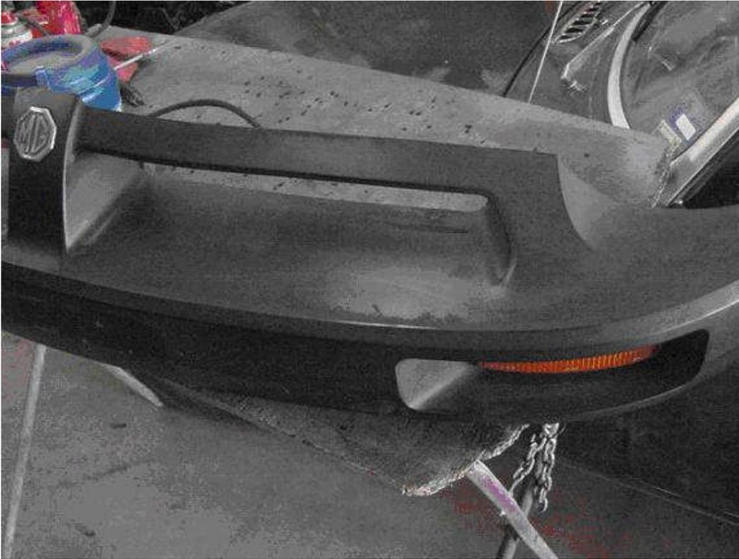
Before any repairs take place. Notice the dull, crazed finish. Home restorers should remove bumpers first
