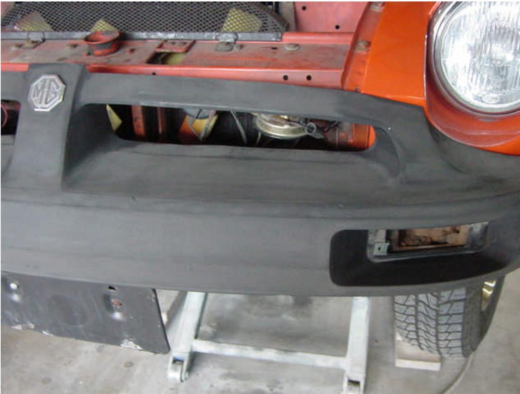
Bumper after cleaning with wax & grease remover and initial sanding
